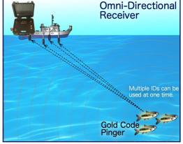
Display real-time direction and depth by calculating the difference of receiving times from 4 receivers
